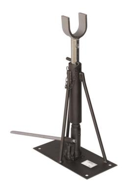
Hydraulic lifting drum stand made of galvanized steel. Composed by a steel structure electro-welded on a flat ground base, a pivot holding head fixed on support shaft with 4 adjustable position, made of galvanized steel, 360° rotating and a support shaft lock pin with chain. Adjustable height by means of hand operated hydraulic piston
